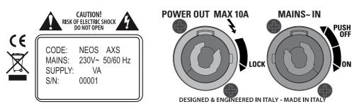
**MAINS IN** - Powercon<sup>®</sup> NAC3FCA power input connector (blue). To switch the amplifier on, insert the Powercon<sup>®</sup> connector and turn it in a clockwise direction into the ON position. To switch the amplifier off, pull back the switch on the connector and turn the connector in an anticlockwise direction into the POWER OFF position.
